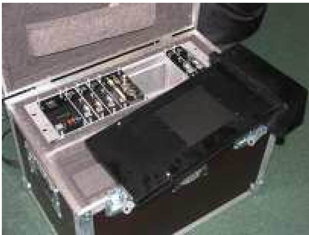
Figure 4. The “Bonn” shutter system for the 10k camera. This custom made shutter (black device) comes with control electronics to fit into a standard rack.
