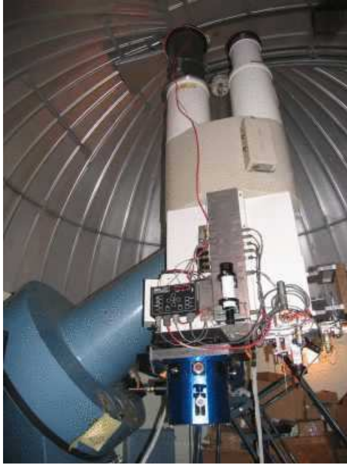
Figure 1. The U.S. Naval Observatory Twin Astrograph, currently at the Flagstaff Station, with 10k camera dewar attached to the “red lens.” This setup will be used for astrometric test observations on the sky in preparation for the URAT program.
